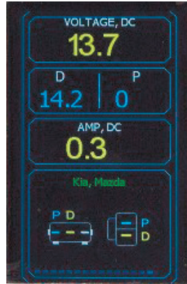
Fig. 13. Display data output when testing a voltage regulator with P-D terminal
