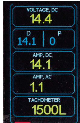
Fig. 6. Display data output when testing an alternator with P-D terminal
