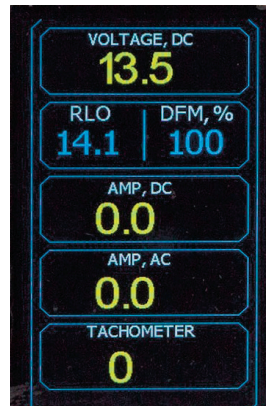
Fig. 8. Display data output when testing an alternator with RLO terminal
