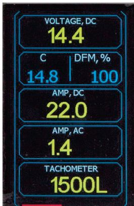
Fig. 7. Display data output when testing an alternator with C terminal
